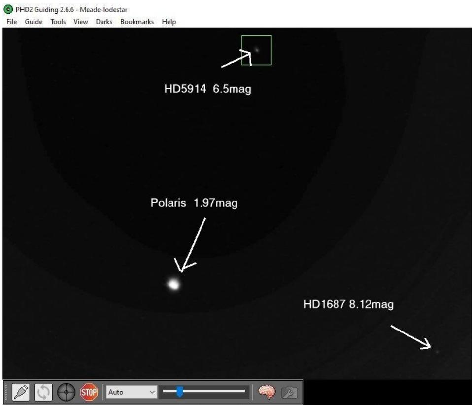
This is a screen grab of PHD2 working with the SV105 camera on a Celestron 70mm Travelscope. Obviously Polaris would make a good guide star. In this case I've selected HD5914, which at 6.5 magnitude is about as dim a star as PHD2 could probably guide on. While HD1685 (8.12 mag) is visible, it is too dim to guide on.
